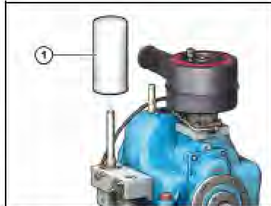
Figure 7-5 Changing the air-oil separating element (sample depiction)
