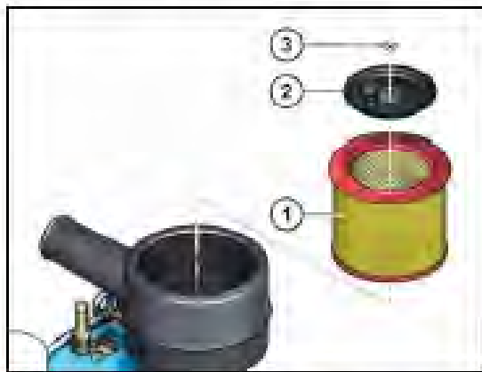
Figure 7-6 Changing the air filter element (sample depiction)
