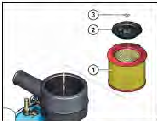
Figure 7-6 Changing the air filter element (sample depiction)
