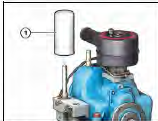
Figure 7-5 Changing the air-oil separating element (sample depiction)
