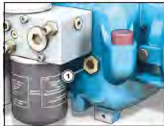
Figure 7-2 Oil level check via sight glass (optional; sample depiction)
