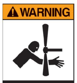
Do not operate without fan guard in place.
