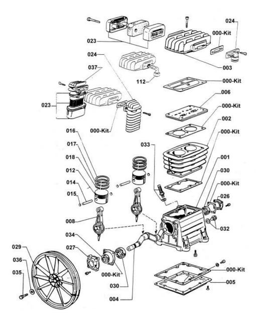
10025-P0098 10025-P0099 10025-P0100 Valve Assembly Kit (#006) Filter (#023) Gasket Kit (#000-KIT)
