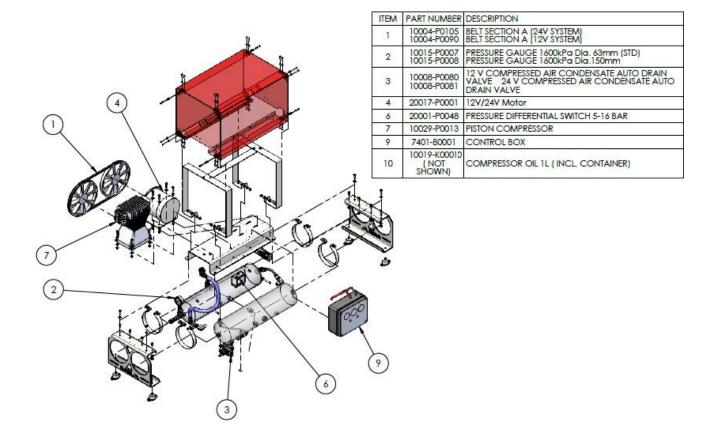
\*Note: Drawing given herein is of fully framed Battery Compressor system. The covers and brackets may not be included in every compressor system package.
