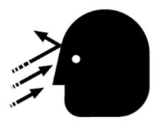
HOT OIL UNDER PRESSURE! Will cause SEVERE PERSONAL INJURY OR DEATH. Do not remove valves, caps, plugs or piping when compressor is running or pressurized. Shut down compressor and relieve system of all pressure before removing valves, caps, plugs or piping 300038
