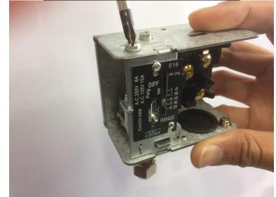
DIFFERENTIAL PRESSURE ADJUSTMENT SCREW (CW TO INCREASE) Adjust to pressure on the gauge as required
