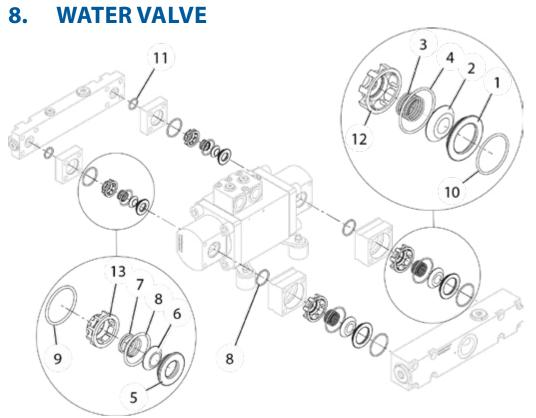
NOTE! The pressure valve's (7) spring has less turns than the suction valve's (3) spring.
