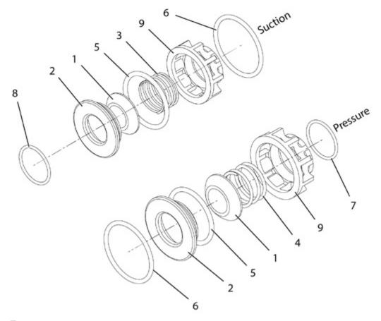
NOTE! The pressure valve's (4) spring has less turns than the suction valve's (3) spring.
