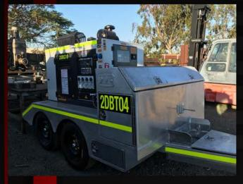
The SMARTWELD 500 AIR has been specifically engineered to meet the highest Australian standards and perform in the harshest environmental conditions. The 3 in 1 - 500 amp Welder, 55 cfm rotary screw Air Compressor and 38 Kva 50Hz generator system, was designed to be fully site compliant with industry regulations.
