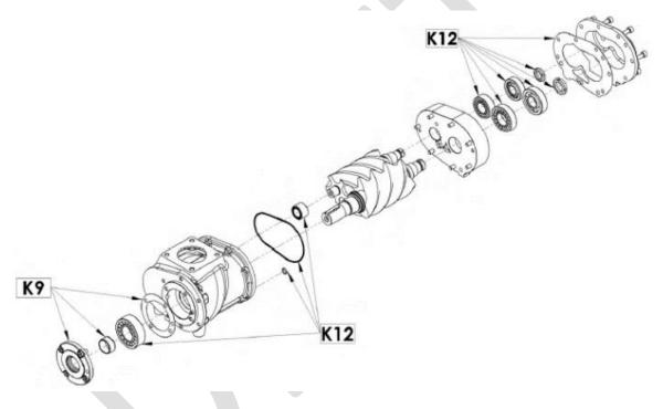
K9-910.0249 Shaft seal spare parts kit K12-910.0248 Bearing spare parts kit
