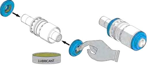
14. Lubricate mating surfaces of the piston assembly and insert it to the body. Place the special tool in the top of the piston assembly.
