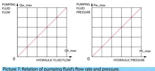
The relation ship between hydraulic oil flow and pressure to pumping fluid flow and pressure is linear.
