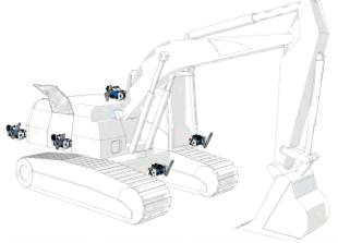
Picture 21: Placing the HDF pump
