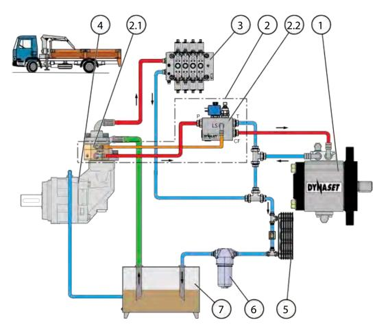
Picture 15: Connection figure for hydraulic system with fixed discplacement pump
