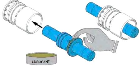
12. Install new o-rings and seals to the sealing flanges. First install o-rings and then the seals. Compress the seal into a kidney shape, place it into groove and push it back to normal shape. Avoid making sharp bends on the seal.
