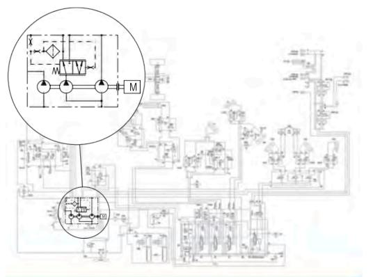
Picture 14: Hydraulic system with fixed displacement pump
