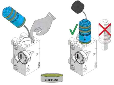
NOTE! Make sure that the piston assembly is installed correctly.
