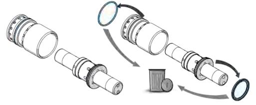
10. Install new o-ring to the cylinder, new o-ring and seal to the piston assembly.
