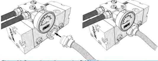
Picture 26: Connection to the pumping fluid intake
