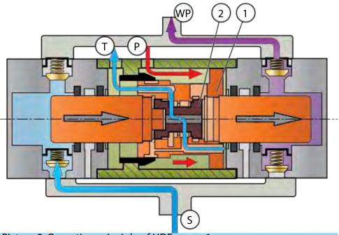
Picture 5: Operating principle of HDF pump 1
