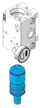
6. Remove the sealing flanges from the piston assembly.
