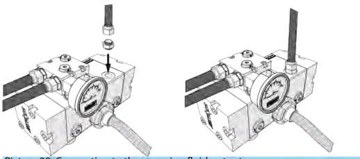
Picture 28: Connection to the pumping fluid output
