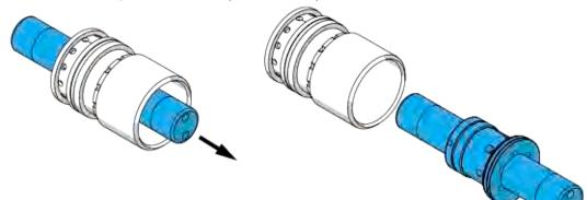
9. Remove seal from the piston assembly and o-ring from the cylinder.
