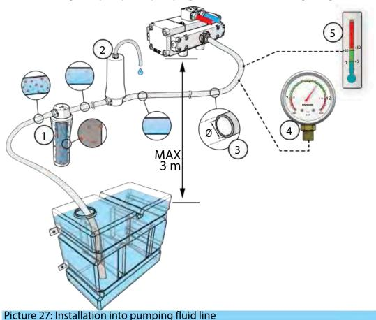
When installing HDF pump into pumping fluid line note following things:
