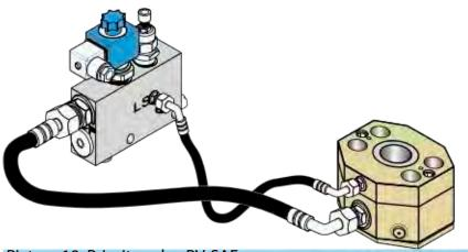
Picture 19: Priority valve PV-SAE
