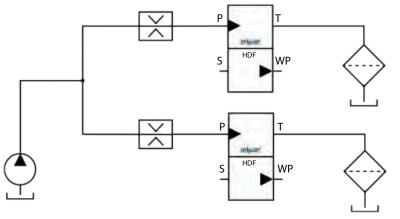
Picture 8: HDF hydraulic line connection in parallel
