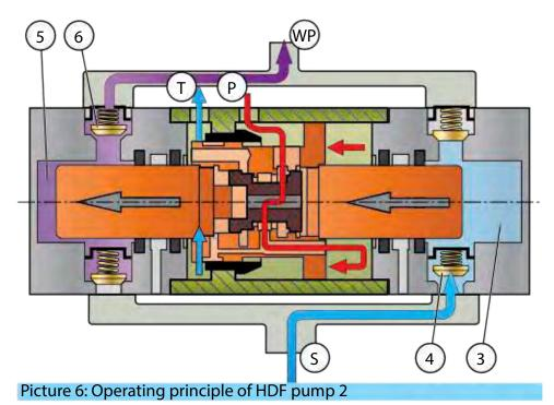
Move of the piston assembly creates pressure and suction. Pump self-primes from water supply line (S) and generates pressure into pressure line (WP). When piston assembly moves away from head it creates underpressure (3) and pumping fluid is sucked through intake valve (4) into head.
