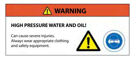
Couplings, valves and hoses need to be kept tight and clean to avoid possible leakages. Leaks in the hydraulic system must be repaired immediately to avoid injuries caused by high pressure blowouts.
