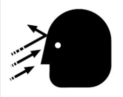
HOT OIL UNDER PRESSURE! Will cause SEVERE PERSONAL INJURY OR DEATH. Do not remove valves, caps, plugs or piping when compressor is running or pressurized. Shut down compressor and relieve system of all pressure before removing valves, caps, plugs or piping
