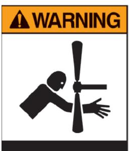
Do not operate without fan guard in place.
