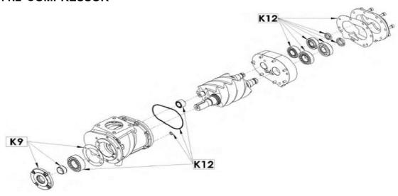
5002-P0002 Shaft seal spare parts kit (K9) 5002-P0004 Bearing spare parts kit (K12)
